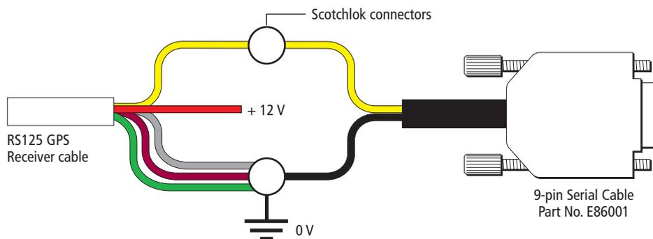
If you are connecting your RS 125 GPS receiver to a PC, you will need a Serial Data Cable, Part No. E86001. Connect the Yellow from the RS 125 to the Yellow of the Serial Data Cable. Connect the Red from the RS 125 to the positive of your boat's 12 V DC power supply. Connect the Brown, Green and Shield from the RS 125 and a Black from the Serial Data Cable to your boat's ground.
