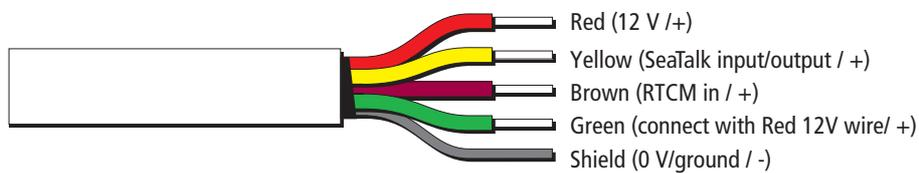
**Note:** If the Brown (RTCM) wire is not used, it must be suitably grounded to 0 Volts.
