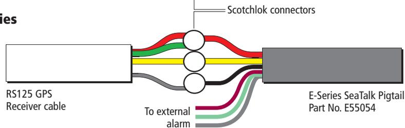
In SeaTalk network installations containing other power devices in addition to your Raystar 125 GPS receiver (e.g. ST series instruments, autopilot controllers, etc.) you should not fix the red wire on your C-Series SeaTalk pigtail to the GPS receiver or overall SeaTalk network.
